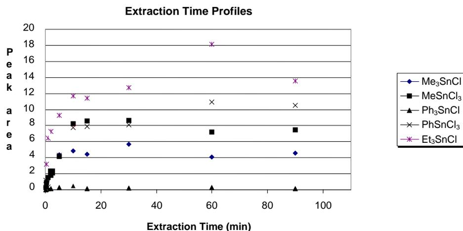
Fig. 2. Headspace extraction time profiles of various tin species (20 µg/l) using 100 µm PDMS fiber.
