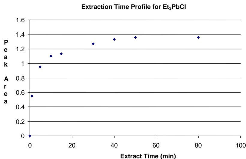
Fig. 3. Headspace extraction time profile of Et<sub>3</sub>PbCl (20 µg/l) using 100 µm PDMS fiber.
