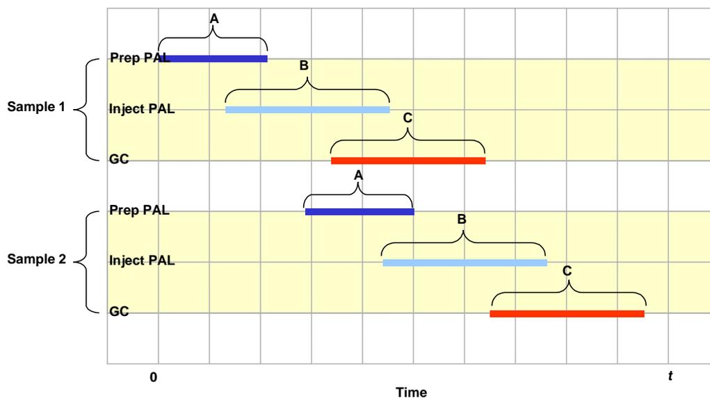
Fig. 4. Time chart of the automated system programmed with Cruise Control 4-2. A = 6 min and 10 s, B = 18 min and 45 s, and C = 18 min and 40 s.
