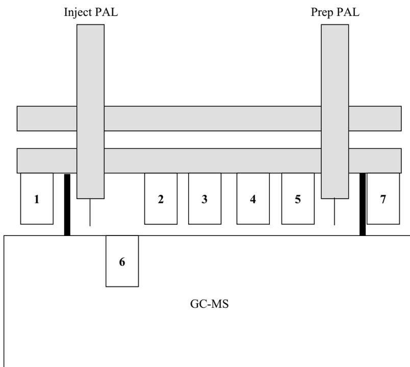
Fig. 1. Drawing of the Twin PAL dual arm system. 1, sample heater/agitator; 2, fiber heater; 3, cooled sample tray; 4, sample tray; 5, fast wash station; 6, GC injector port; and 7, sample heater/agitator 2.
